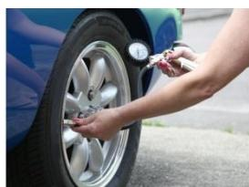
Car Tyres: As cars are driven the friction between the tyres and the road causes the air inside the tyres to heat up. This means that the particles of air are moving more quickly and hitting the insides of the tyre with more force and more often. Since the volume of the inside of the tyre does not change the pressure of the air inside the tyre rises.
