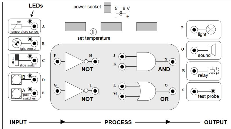
This circuit turns on central heating automatically when the system is turned on with the slide switch, C, and the temperature in the room becomes low. The circuit makes use of a motor connected to the relay to operate the pump in the central heating system. The combined truth table for the circuit would be:
