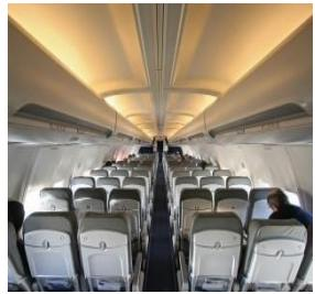
Aircraft cabins: When an aircraft flies at a high altitude, the atmospheric pressure outside the cabin is very low. In fact, the pressure is so low that if the pressure inside was the same as outside it would lead to altitude sickness in all of the passengers and crew. To avoid this happening, extra air is pumped from outside into the cabin, increasing the pressure inside and simulating the pressure we experience at ground level.
