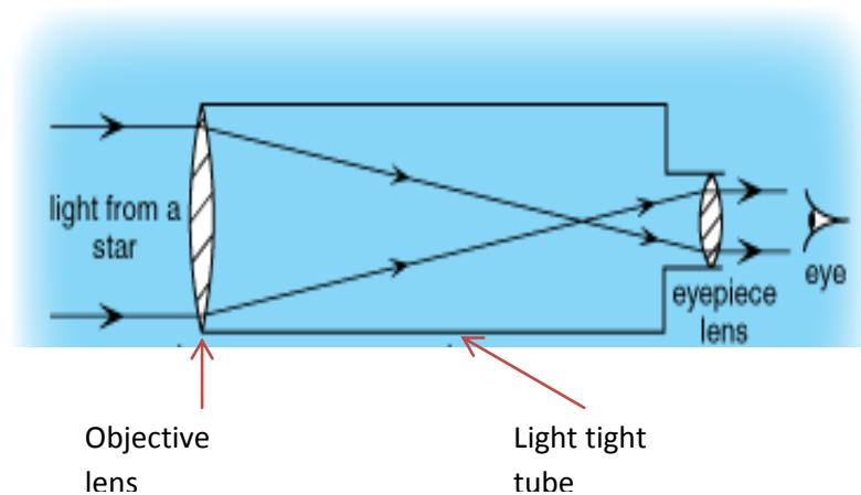
Refracting telescopes use lenses to obtain images of distant objects. A refracting telescope consists of an **objective lens**, an **eyepiece lens** and a **light tight tube**. The objective lens produces an image which is then magnified by the eyepiece lens and the light tight tube cuts out light from other sources. The larger the diameter of the objective lens the more light it can collect and therefore the brighter the image.
