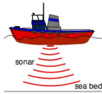
Ultrasound waves can also be used to measure the depth of the ocean and to monitor fish numbers. The time taken for the sound to reflect can be used to calculate the depth of the ocean. The speed of sound in water is much higher than it is in air because the particle's in the water are much closer together than they are in the air. Ultrasound which is used in this way is often called sonar.
