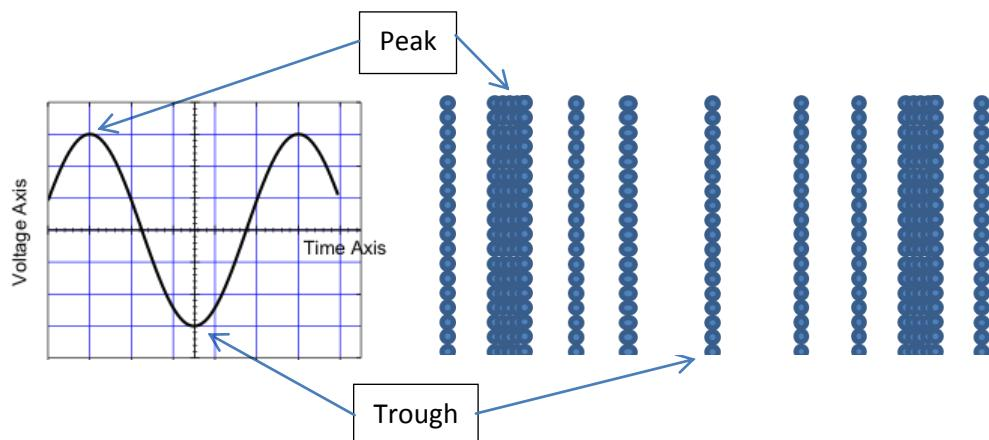
The more peaks and troughs that are shown on the oscilloscope trace the higher the frequency and pitch of the sound.
