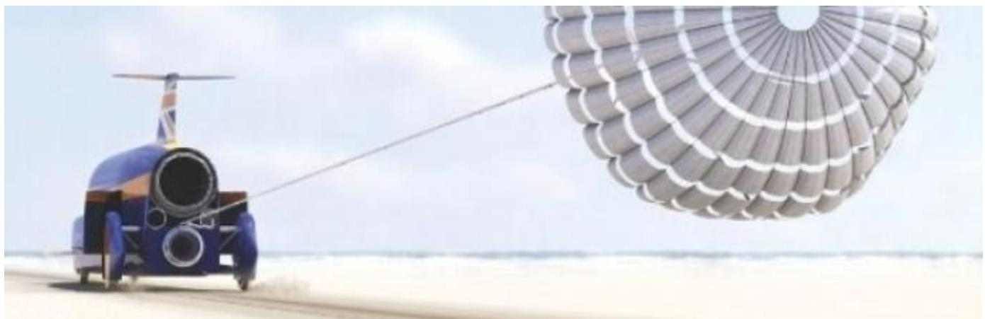
Bloodhound SSC has three primary braking systems: airbrakes, parachutes and wheel brakes. These will be used one-by-one to slow the car down from its top speed of over 1,000mph, taking advantage of the inherent benefits of each one:
