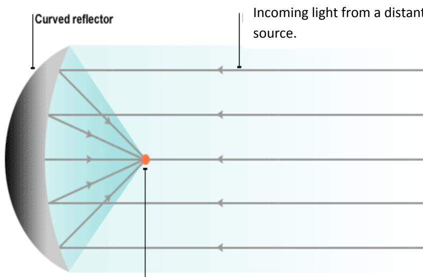
Curved reflectors are used to reflect light to increase the brightness of the image of a distant star or other source. The curved shape of the reflector collects the light from over a large area and brings it to a focus. The detector of light is placed at the focus so that it receives a brighter image.
