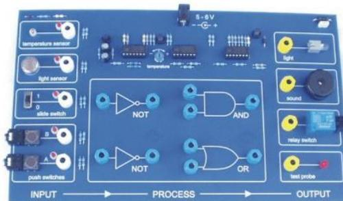
The **temperature sensor / thermistor** is used in circuits where detecting temperature is important such as a thermostatically controlled central heating system. As the temperature of the sensor rises its resistance decreases. This causes a change in the signal given out from the input device that is being passed to the process device. When the sensor is warm it is described as giving out a “logic 1” signal but when the sensor is cold it gives out a “logic 0” signal.
