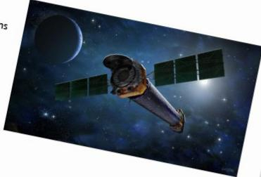
X-ray telescopes can see high temperature explosions in space but can only be used when placed in space because the Earth's atmosphere will absorb X-rays. Having telescopes in space is expensive to set up, as well as to repair and maintain.
